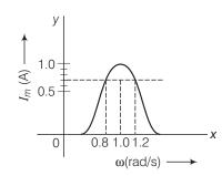
where  $\omega_1$  and  $\omega_2$  corresponds to frequencies at which magnitude of current is  $\frac{1}{\sqrt{2}}$  times of maximum value.
