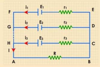
$$I = \frac{\sum_{i=0}^{n} \frac{E_{i}}{r_{i}}}{1+R\sum_{i} \frac{1}{r_{i}}} \text{ and } E_{eq.} = \frac{\sum \frac{E_{i}}{r_{i}}}{\sum \frac{1}{r_{i}}}, r_{eq.} = \frac{1}{\sum \frac{1}{r_{i}}}$$
