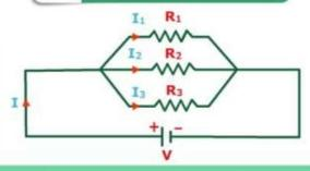
The sum of current passing through each resistance is equal to the total current coming from the battery.
