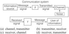
5. If the output of the information source is a nonelectrical signal like a voice signal, a ..... converts it to ..... form before giving it as an input to the ......
