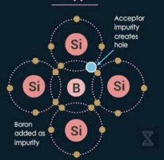
When impurity of 3rd group is added in an intrinsic semiconductor, then P-type semiconductor is formed.
