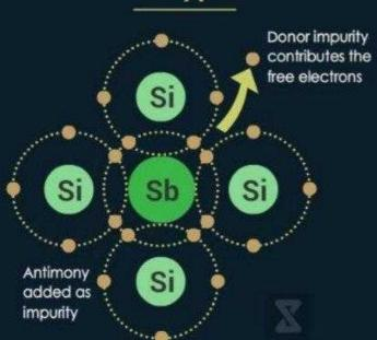
When impurity of 5th group is added in an intrinsic semiconductor, then N-type semiconductor is formed.
