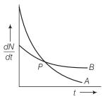
We know that  $\left(\frac{dN}{dt}\right) \propto \lambda_{A}$ , at any instant of time hence we can say that  $\lambda_{A} > \lambda_{B}$ . At point *P* shown in the diagram the two curve intersect.
