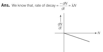
where decay constant ( $\lambda$ ) is constant for a given radioactive material. Therefore, graph between *N* and  $\frac{dN}{dt}$  is a straight line as shown in the diagram.
