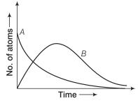
At t = 0,  $N_A = N_0$  (maximum) while  $N_B = 0$ . As time increases,  $N_A$  decreases exponentially and the number of atoms of *B* increases. They becomes ( $N_B$ ) maximum and finally drop to zero exponentially by radioactive decay law.
