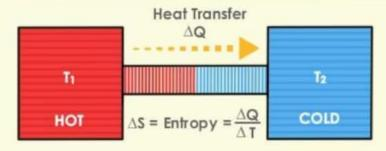
This law states that energy naturally flows from hotter objects to cooler objects. In order for energy to flow from a cooler object to a hotter object, work must be done. When heat is converted into work, the efficiency or output of usable work will always be less than 100%.
