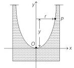
Pressure at any point P due to rotation is
