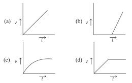
**143** Which of the following diagram does not represent a streamline flow?
