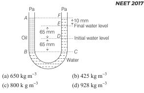
**16** Find density of ethyl alcohol. Using information given in the diagram below **JIPMER 2018**
