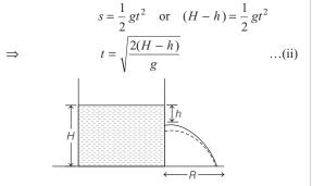
The distance *R*, where the emerging stream strikes the floor is given by R = vt
