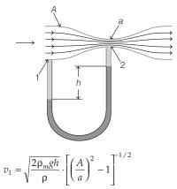
where,  $\rho_m$  = density of liquid contained in U-tube,  $\rho$  = density of fluid
