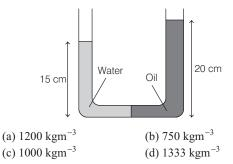
**15** A U-tube with both ends open to the atmosphere is partially filled with water. Oil which is immiscible with water, is poured into one side until it stands at a distance of 10 mm above the water level on the other side. Meanwhile the water rises by 65 mm from its original level (see diagram), the density of the oil is
